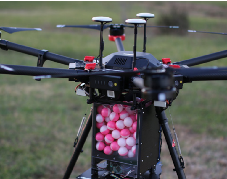
FIGURE 22: A drone equipped with IGNIS incendiary balls. Credit: Drone Amplified.
